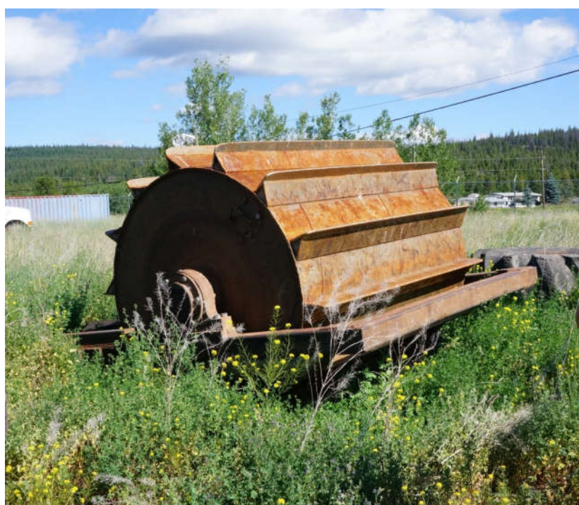
Figure 7. Example of a roller–chopper machine for treating postharvest debris.
